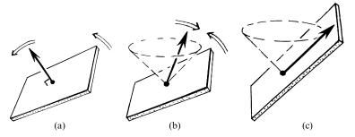
**Fig. 18.5** (a) In Euclidean 4-geometry, if a direction rotates, so also does its orthogonal complement 3-plane element. (b) This is true also in Lorentzian 4-geometry, but for a timelike direction the slope of the orthogonal complement 3-plane (spatial directions of 'simultaneity') moves in the reverse sense; (c) accordingly, if the direction becomes null, the orthogonal complement actually contains that direction.
