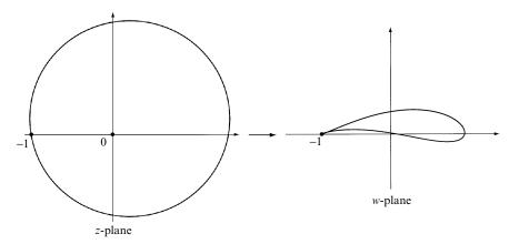
**Fig. 8.15** Zhoukowski's transformation  $w = \frac{1}{2}(z + 1/z)$  takes the exterior of a circle through z = -1 to an aerofoil cross-section, enabling the airflow pattern about the latter to be calculated.
