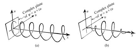
**Fig. 21.5** A particle wavefunction:  $\psi$  as a complex function of position x. (a) Momentum state  $e^{-iPx/\hbar}$ , depicted as a corkscrew (eigenfunction of momentum p). (b) A wave packet  $e^{-A^2x^2}e^{-iPx/\hbar}$ .
